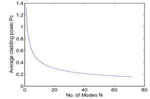
Figure 5. Variation of average cladding power  $\left(P_{c}\right)$  with number of modes (N)
