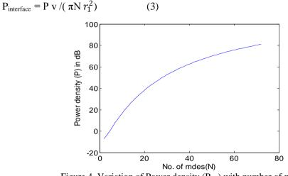
Figure 4. Variation of Power density (P<sub>dB</sub>) with number of modes
