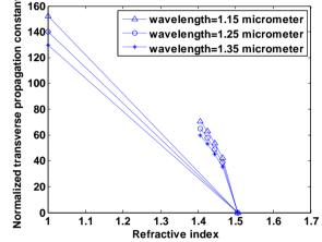
Figure 2: Variation of normalized transverse propagation constant with n of each layer.
