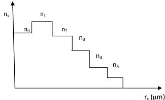
Figure 1: Variation of refractive index  $(n_x)$  with the number of cladding layers of optical fiber.
